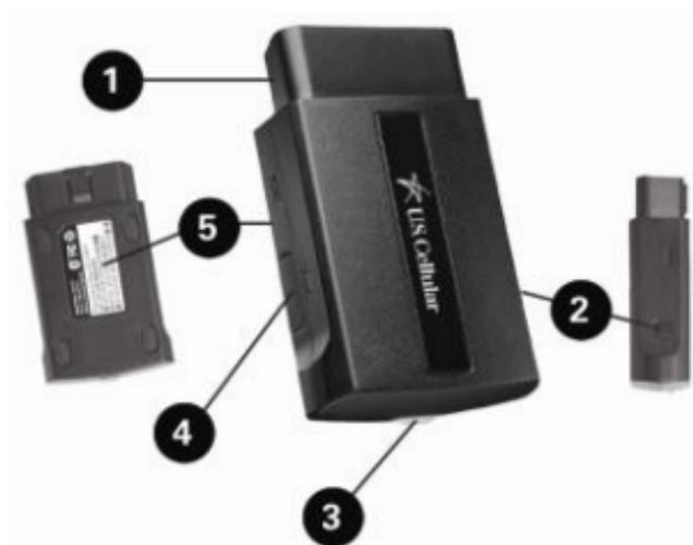
1. OBD connector (plugs into vehicle 's OBD port)
